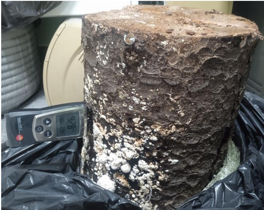
Fig. 2 – Measuring the timber absolute moisture content with a moisture meter Testo 606-2
