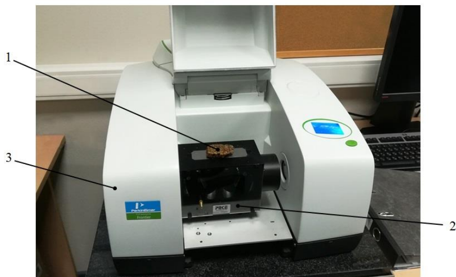
Figure 2 - General view of the installation for determining the optical characteristics of the honeycombs: 1 - sample; 2 - cuvette; 3 - IR - Fourier spectrometer.
