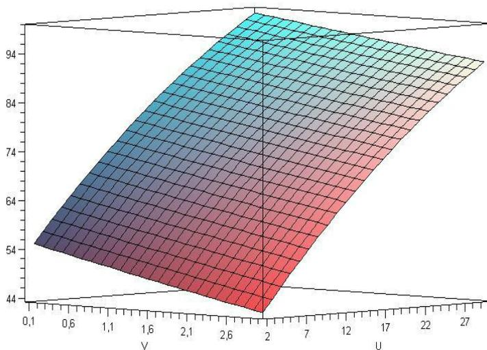
Figure 3 – The surface of the response function with varying parameters:  $V$  – air velocity;  $U$  – voltage on the electrodes at a fixed value of  $n = 500$  (upper level)
