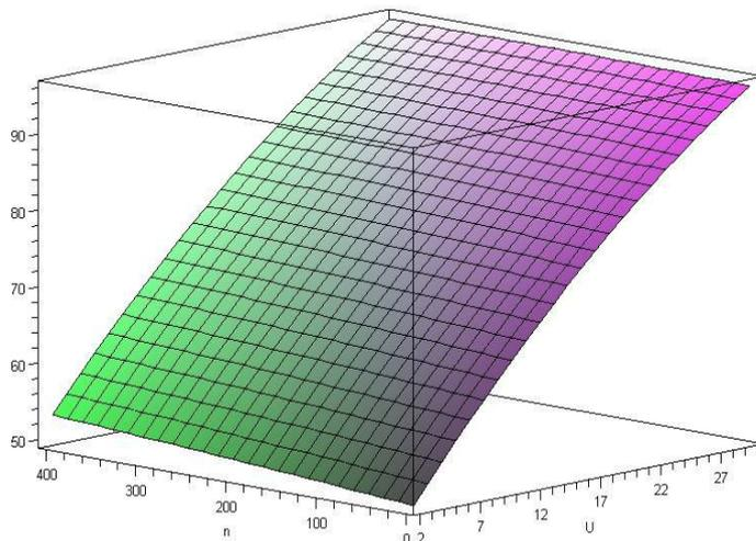
Figure 1 – The surface of the response function with varying parameters:  $U$  – voltage;  $n$  – pulse frequency at a fixed value of  $V = 1.75$  (centre of the experiment)
