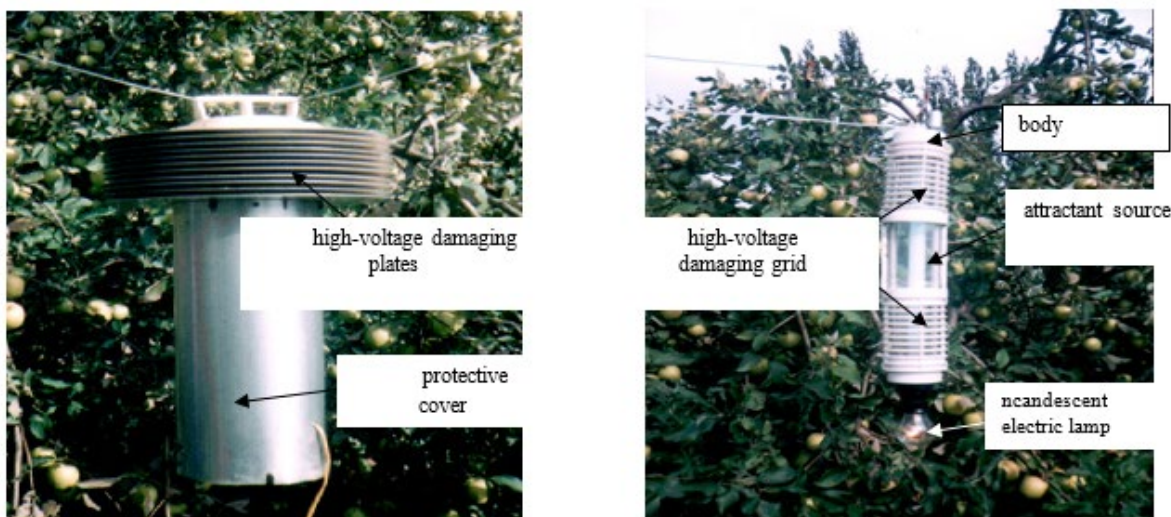
Figure 2 – Types of designs of electro-optical converters with high-voltage damaging element
