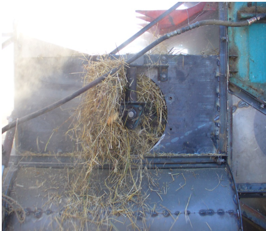
Figure 1 – Removal of chopped straw by the auger in the harvester stacker installed on the "Enisey – 1200R" combine harvester
