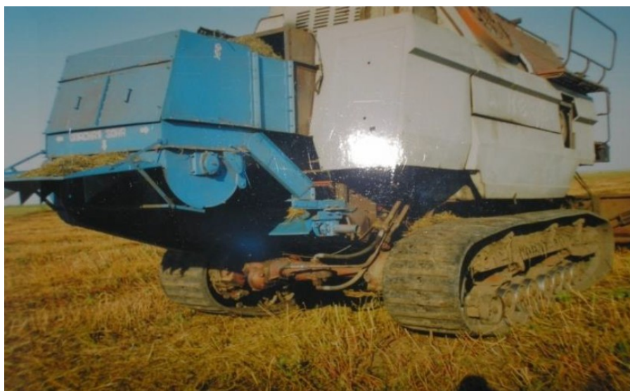
Figure 3 - Grinder - spreader - straw roller "IRVS-1200" in the aggregate with the grain harvester "SZK - 1200 RAG" DOI: https://doi.org/10.60797/JAE.2026.65.3.6
