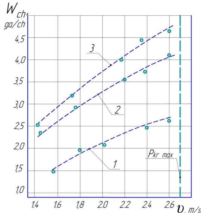
Figure 5 – The Dependence of the hourly productivity of  $W_{ch}$  on the speed  $v$  of movement of the arable unit: 1-K-701 + PNL-8-40; 2-K-701+PBS-8M; 3-K-701+PBFR-5.  $P_{kr}$ -the maximum pulling force of the tractor K-701
